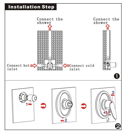
**\*** Read the Installation Fig and confirm the installing position.
